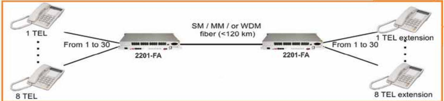
1 - 30 FXS to 1 - 30 FXS configuration, clear channel
