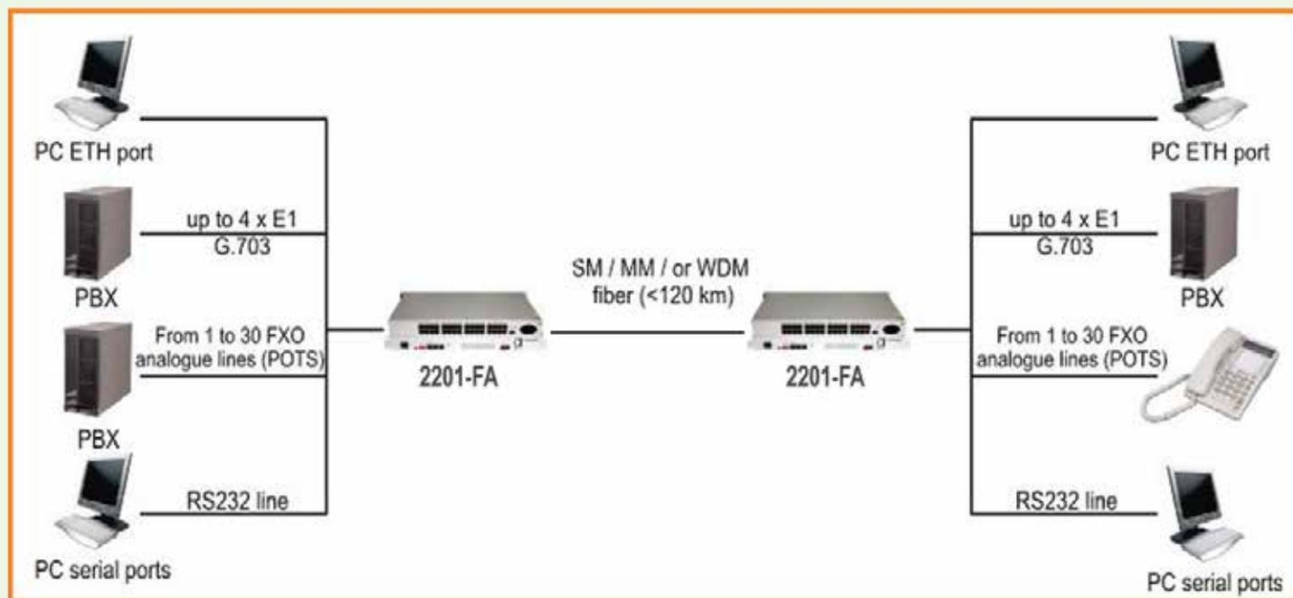
Full connection scenario, where all possible connections are used - 30 FXS/FXO, RS-232, Ethernet and 4E1
