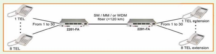
1 - 30 FXS to 1 - 30 FXS configuration, clear channel
